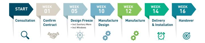
Figure 3.4: Greenstone.ie – Off-site Manufacturing Value Chain Process Map for Residential Modular Construction (Ref: https://greenstone.ie/?page\_id=96)
